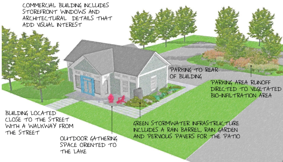
Figure 4-2. Building Placement and Design Standards Illustrated
