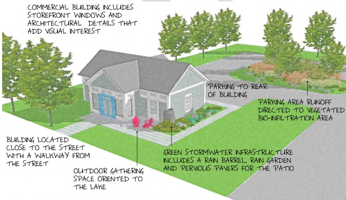
Figure 4-2. Building Placement and Design Standards Illustrated
