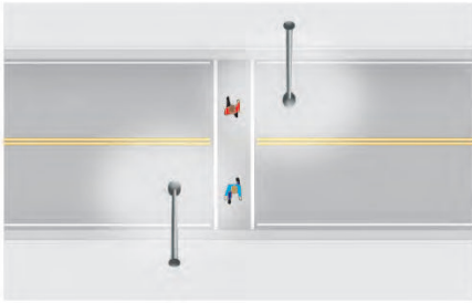
Proper placement of crosswalk illumination (Credit: Michele Weisbart)
